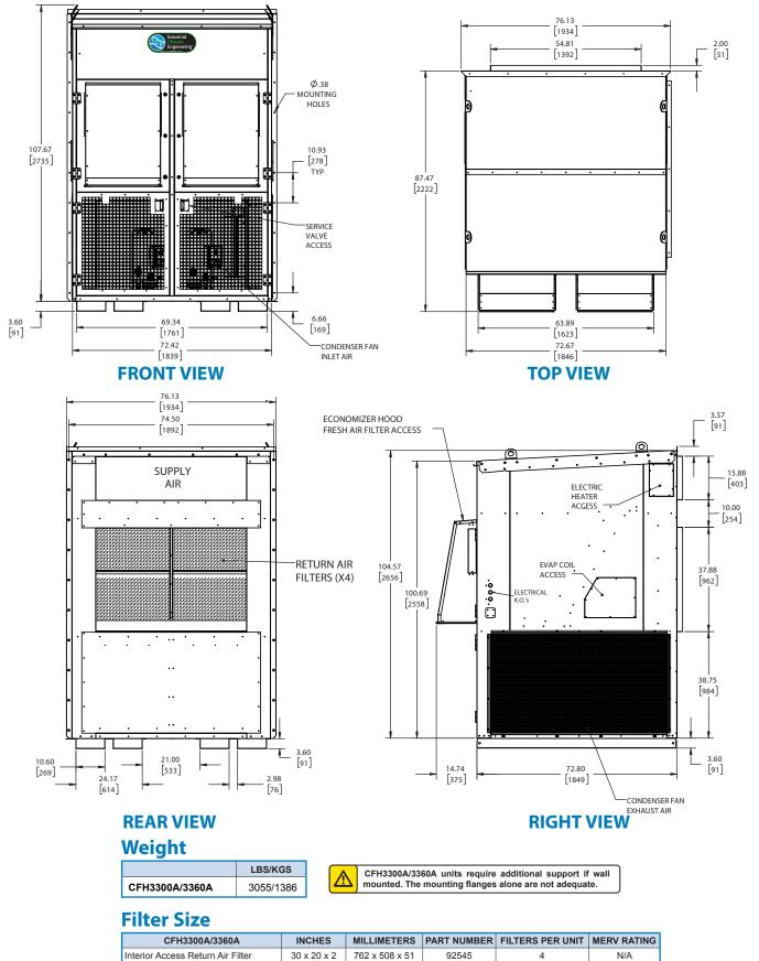
Fresh Air Filter (Economizer Only) 92982 15 x 26 x 1 381 x 660 x 25 2 Note: All overall outside dimensions are given with +/- .250" (6mm) tolerance.
