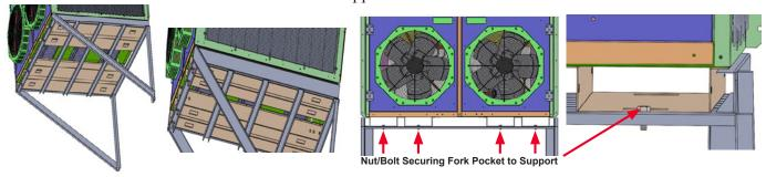
Figure 6a Unit Compression Support Examples
