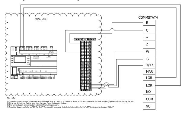
Figure 7b. CommStat 4 Connection Diagram
