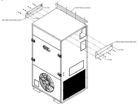
Figure 3. Top Flange and Lifting Bracket Installation (Typical)
