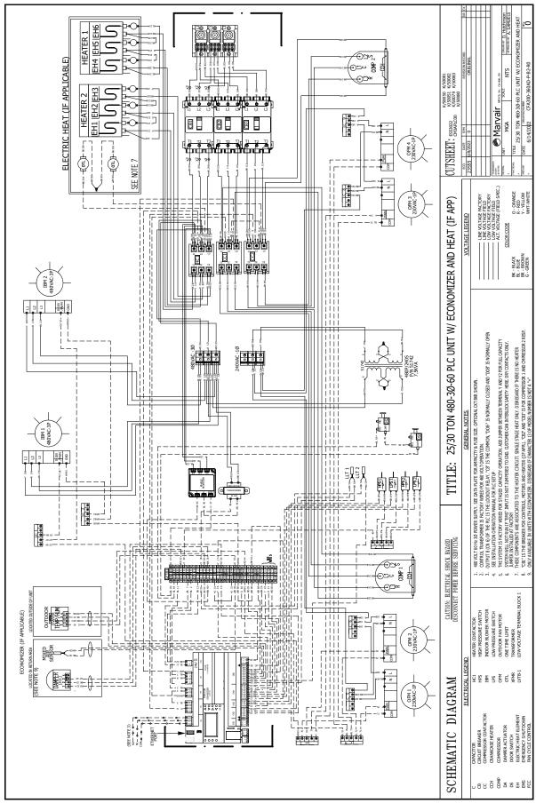
Figure 2b. Typical Electrical Schematic - CFH3300A & CFH3360A
