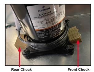
Figure 5. Compressor Chock Removal
