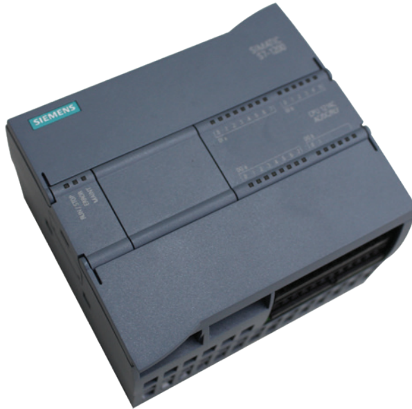
Figure 1. Programmable Logic Controller
